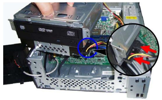
8. Connect one end of the SATA cable to the SATA connector on the mainboard.
